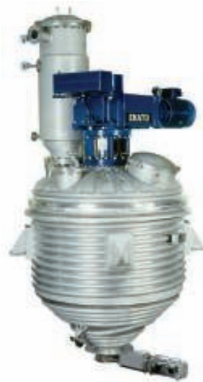
FIGURE 3. Vertical solids dryers can take advantage of gravitational forces for solids flow
