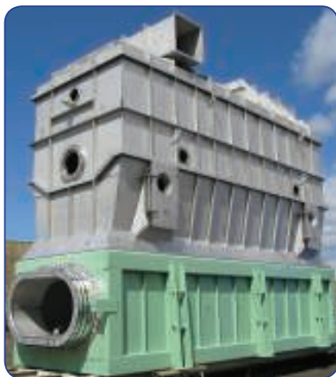
Attention to airflow and thermal expansion lets GEA create fluidized beds up to 100 m 2
